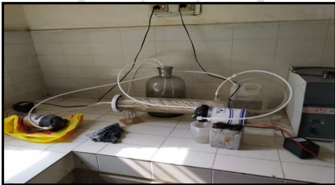
Figure 3 Forward Osmosis (FO) set-up
