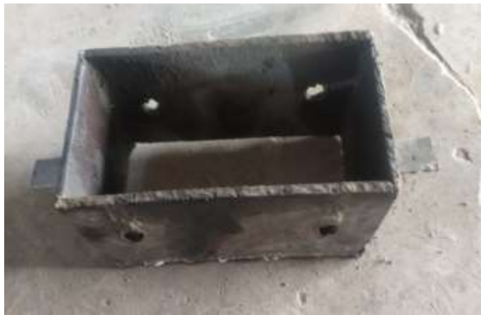
Figure – Mould sample for interlocking block.
