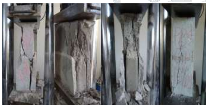
Figure: Compressive strength test of interlocking block.
