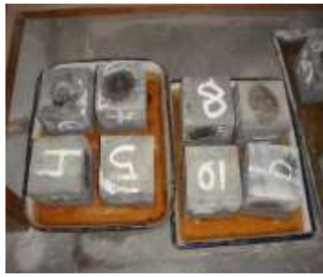
(a) Mortar of Geo-polymer concrete block
