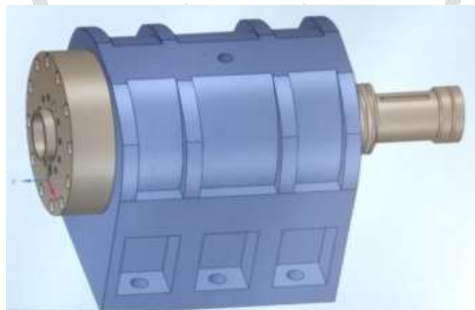
Figure 19 CAD Model for spindle housing system
