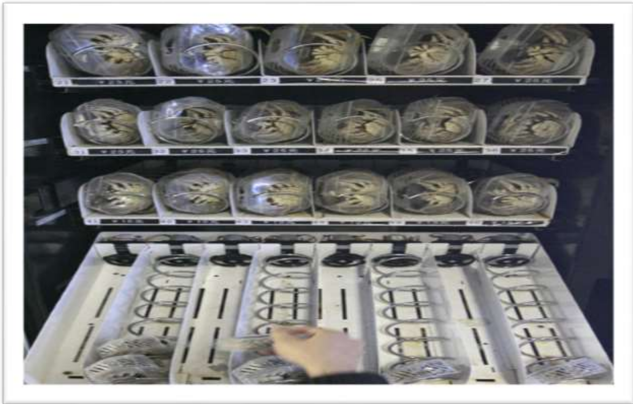
Figure 3.2: Squeeze mechanism (Archimedes' screw) in vending machine.
