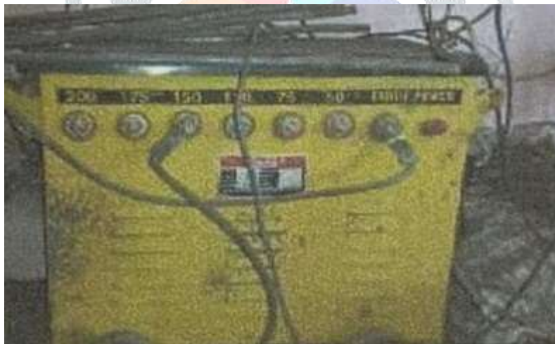
Figure 2: Basic SMAW setup.
