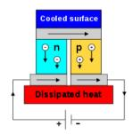
When an electric current is passed through a circuit of a thermocouple, heat is evolved at one junction and absorbed at the other junction. This is known as the Peltier Effect. The Peltier effect is the presence of heating or cooling at an both the side.
