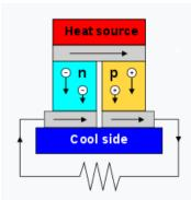
A thermoelectric circuit composed of materials of different Seebeck coefficients (p-doped and n-doped semiconductors), configured as a thermoelectric generator. If the load resistor at the bottom is replaced with a voltmeter, the circuit then functions as a temperature-sensing thermocouple.
