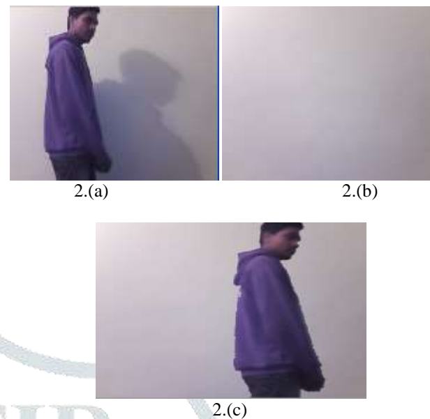
Fig.2. Background subtraction and shadow removal (a)Video Frame, (b)Background Subtraction, (c)Remove Shadow
