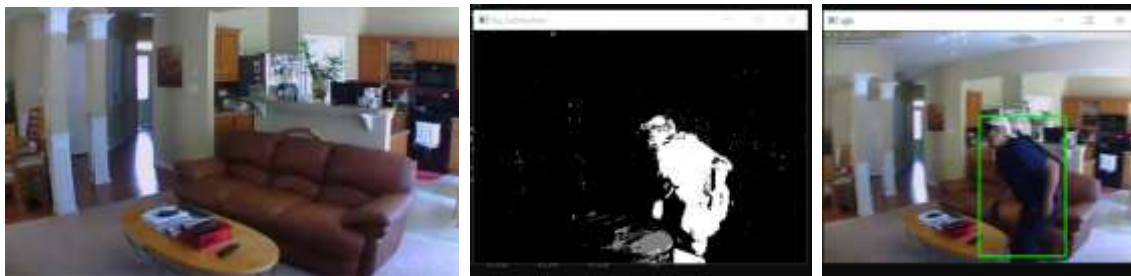
Figure 2: Representational analysis of background extraction, background subtraction and object tracking.
