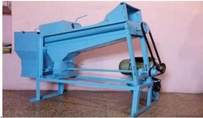
Fig.1. Actual fabricated model of corn peeling and cutter machine
