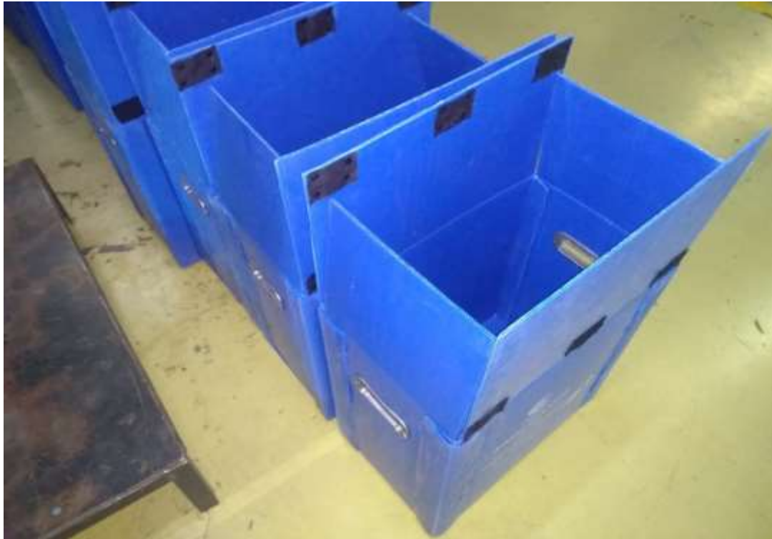
Fig.5.1.Welded PP box ( Final Result)
