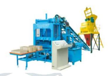
The machine produces blocks and bricks of stable and high quality with a low rate of waste products. The device employs electronic, hydraulic, and mechanical integrated technology, and each program can lock each other. Thus, the whole process is connected smoothly. The machine is versatile. Hence, it can produce various types of porous blocks, standard bricks, hollow blocks, paving blocks, curb stone grassland bricks, and so on by changing the individual moulds.
