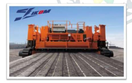
The powerful Volvo TAD721VE watercooled engine, with high-torque reservation, low fuel consumption, and emission, European environmental conforms to standards. They are also fitted with an original German water cooling engine with reliable and robust power. The Control System Micro-computer system with selfdiagnostic capability. Hydraulic synchromesh for vibration bar contains the step-less frequency conversion to supply optimum frequency for all kinds of concrete works.
