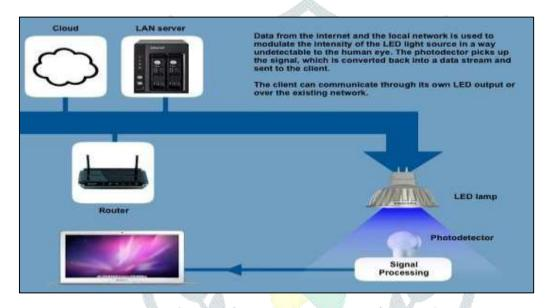
To further get a grasp of Li-Fi consider an IR remote. It sends a single data stream of bits at the rate of 10,000-20,000 bps. Now replace the IR LED with a Light Box containing a large LED array.
