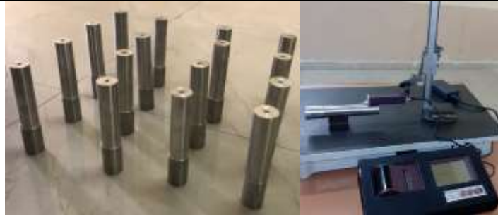
Fig.4 AISI 316L workpiece after machining and surface roughness tester SJ-301
