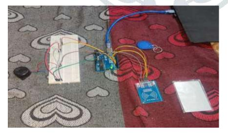
We have made one small prototype of RFID system which is to be applied in the industry. In this prototype we have used Arduino, RFID reader, RFID tags, Breadboard, jumper wires, LEDs and buzzer. Connections are made with the help of connection diagram in the fritzing software. For programming purpose we have used Arduino IDE software which makes good communication with Arduino UNO. Program is attach in the appendix.
