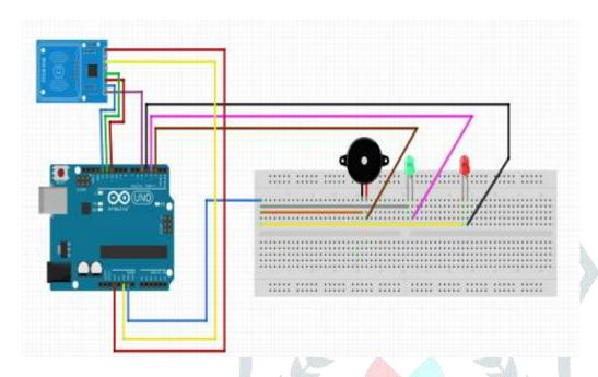
The connection diagram is drawn by using fritzing software. It is easily available on internet for drawing these kind of project diagrams. By using this software we get idea regarding how to make connections for accurate working of this prototype. Figure shows connections of this prototype and also required components.
