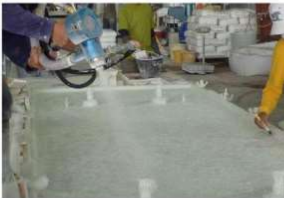
figure:-1 spray-up method
