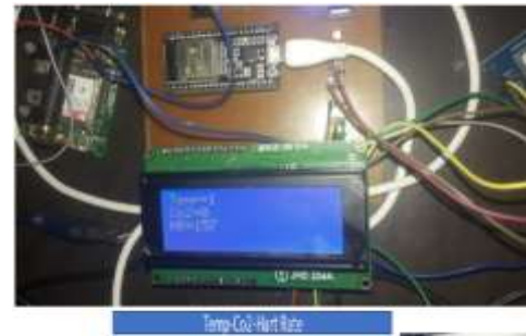
Figure 13. Temperature, oxygen, heart rate sensor results on LCD screen
