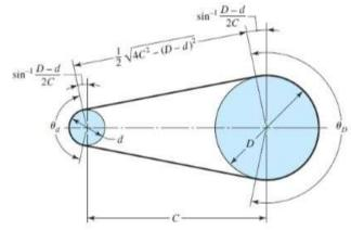
The angle of contact in the driven and driver roller:
