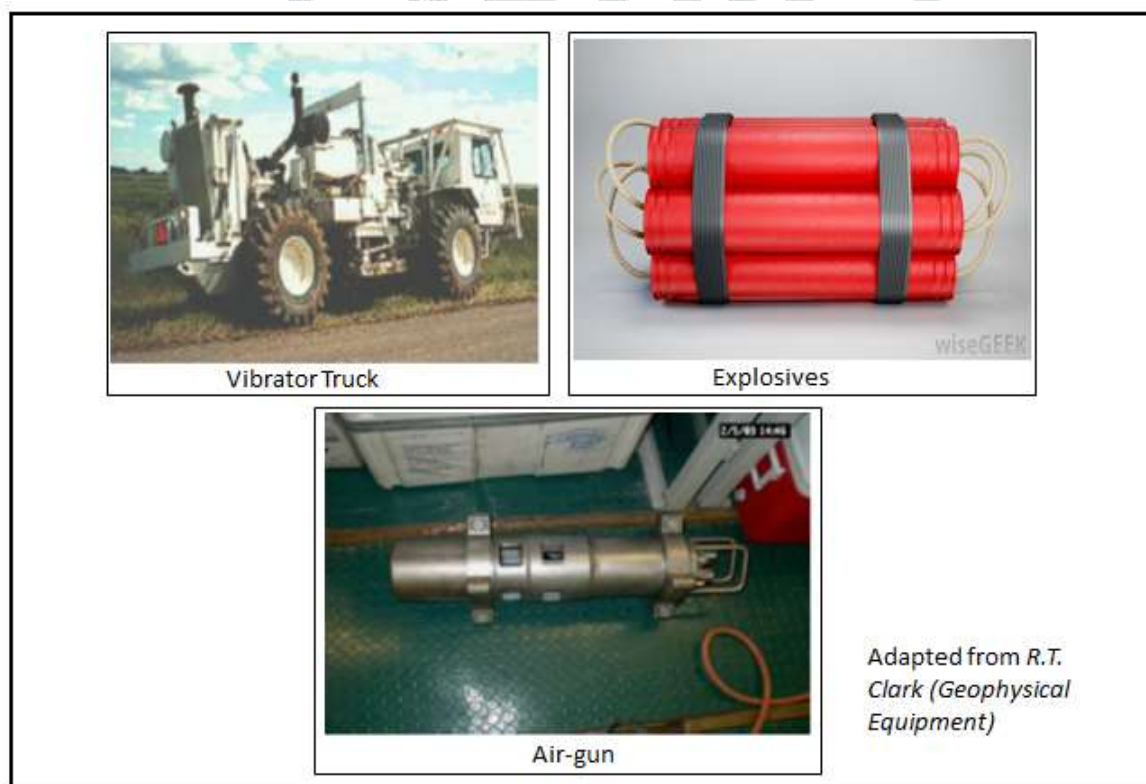
Figure 1:- different types of sources used in seismic data acquisition
