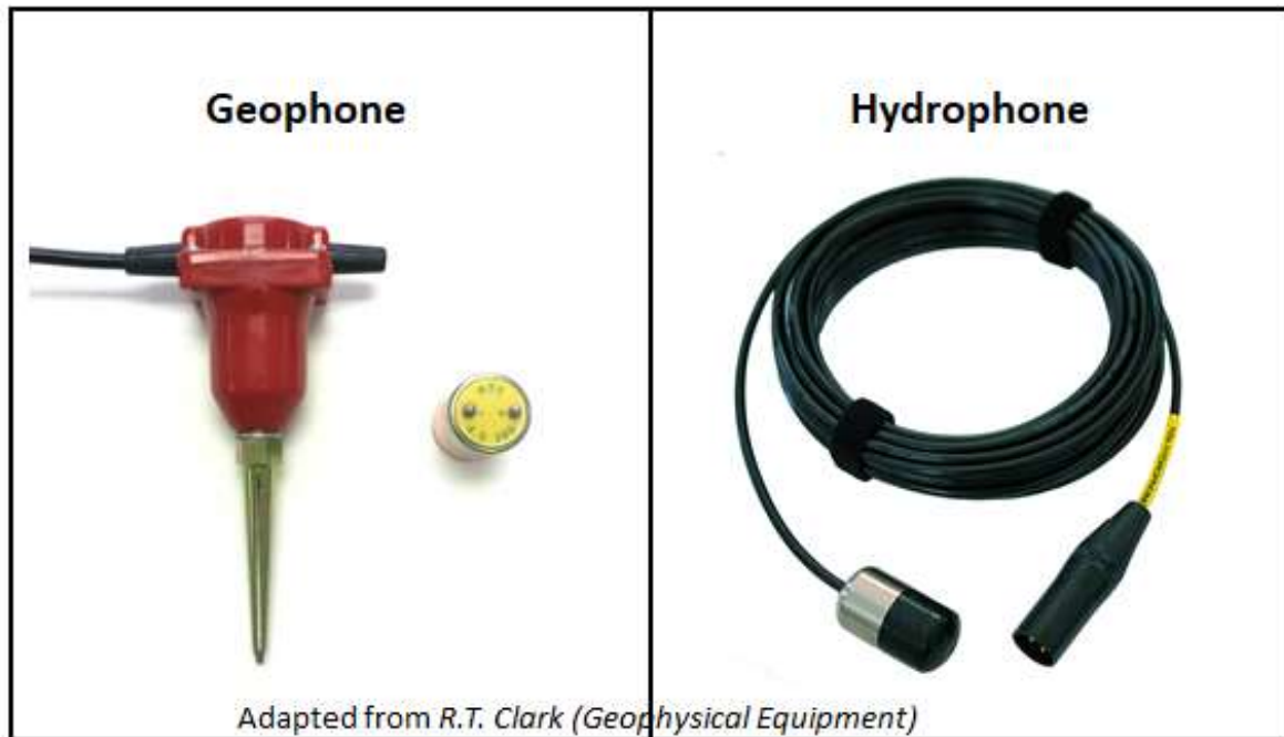
Figure 2: receivers used onshore ( geophone ) and offshore ( hydrophone ) in seismic data acquisition
