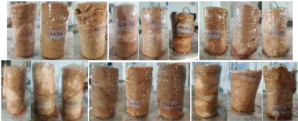
Fig. 6 Failure pattern of Carbonate rock matrix
