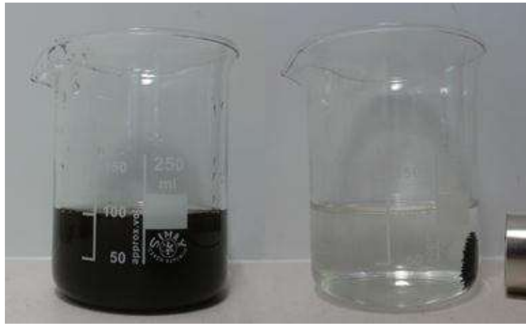
Fig. 1 Demonstration of magnetic properties of prepared iron oxide nanoparticles dispersed in water
