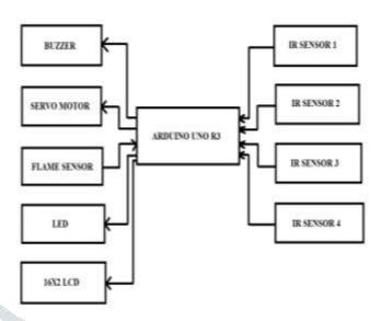
Fig 3: -Block Diagram for Person Counter & automatic lights
