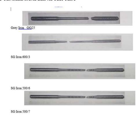
The above test samples are used to measure tensile, yield and elongation under universal test mechanic for different groups of materials grade, refer figure ----- which is belongs to grey iron not having deformation at the fracture end.
