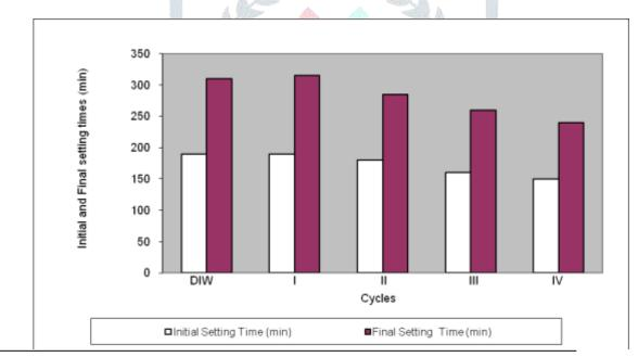
Fig. 4.3. Comparison between Cycles and Initial and Final Setting times
