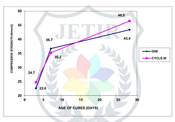
Fig 4.6. Variation of compressive strength for DIW and Cycle III
