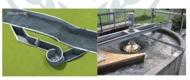
SCREW TURBINE (Reverse Archimedes' screw): two low-head schemes in England, Settle Hydro and Torrs Hydro use an Archimedes' screw which is another debris-tolerant design. Efficiency 85%.
