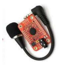
The Voice Recognition Module is a compact and easy-to-control speaking recognition board. Voice Recognition Module is a speaker-dependent voice recognition module. It supports 80 voice commands in total. Any sound can be directed as a voice command. This board has 2 control methods: serial port (full function), common input pin (part of function).
