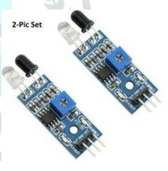
The sensor consists of two diodes, one diode sends out infrared light and the other diode receives the light reflected from the surface. When infrared rays fall on a white surface, they are reflected back and when infrared light.
