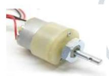
Geared DC motor is in fact an ordinary dc motor with metal speed reduction gears combined on purpose to scale down its rotation per minute (RPM) rate.
