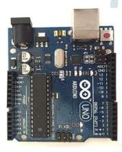
Raspberry Pi does not provide ADC (Analog Digital Converter) on its chip. This limits the Raspberry Pi if you want to use a non digital sensor. So, we are using Arduino to control every moment.
