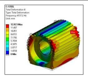
Fig. Mode shape 6 with natural frequency of 4137.2 Hz
