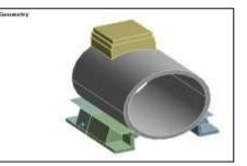
Fig Geometry of motor casing
