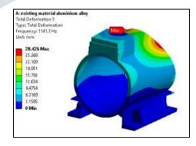
Fig. Mode shape 5 with fundamental frequency 1141.3 Hz
