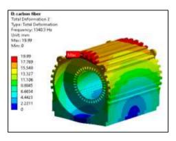
Fig. Mode shape 2 with natural frequency 1340.3 Hz
