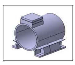
Fig.1 CATIA model of motor casing
