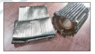
Fig. Motor housing with carbon fiber
