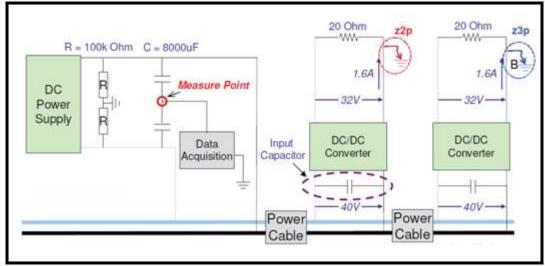
Fig.4. Ground fault detection system for ungrounded DC system [5]
