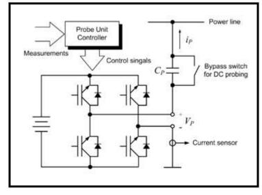
Fig.1. A schematic of probe unit using full-bridge inverter that can generate voltages with arbitrary amplitude and frequency [1]
