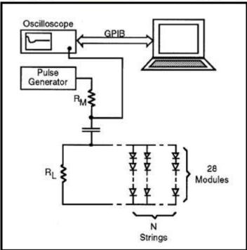
**Fig.2.** Step excitation voltage based approach [2]
