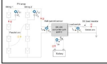
Fig.6. Circuit diagram and arc generation setup in solar PV system [8]
