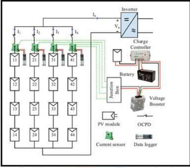
Fig.5. Solar PV fault analysis system model set up [6]
