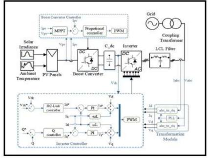
Fig.7. Control structure of the GCPV system [10]
