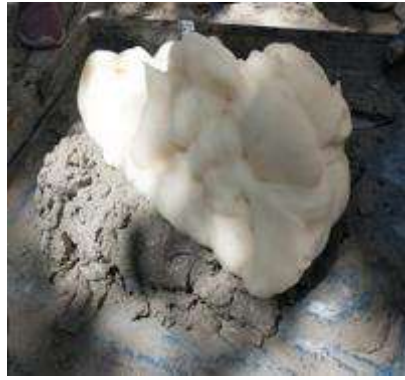
( Figure 2 : Mixing of Foam Concrete )
