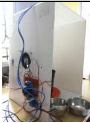
Fig.7.The PCB fitted on right side of enclosure
