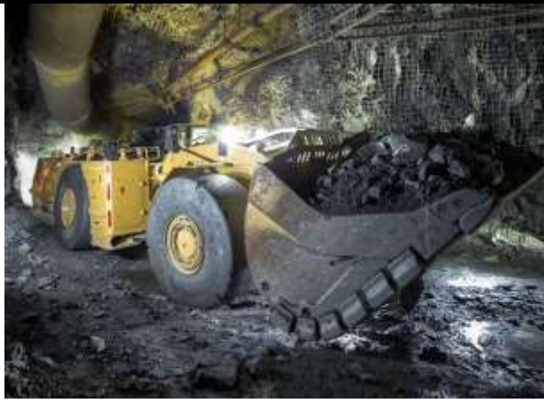
Fig.6: Load haul dumper
