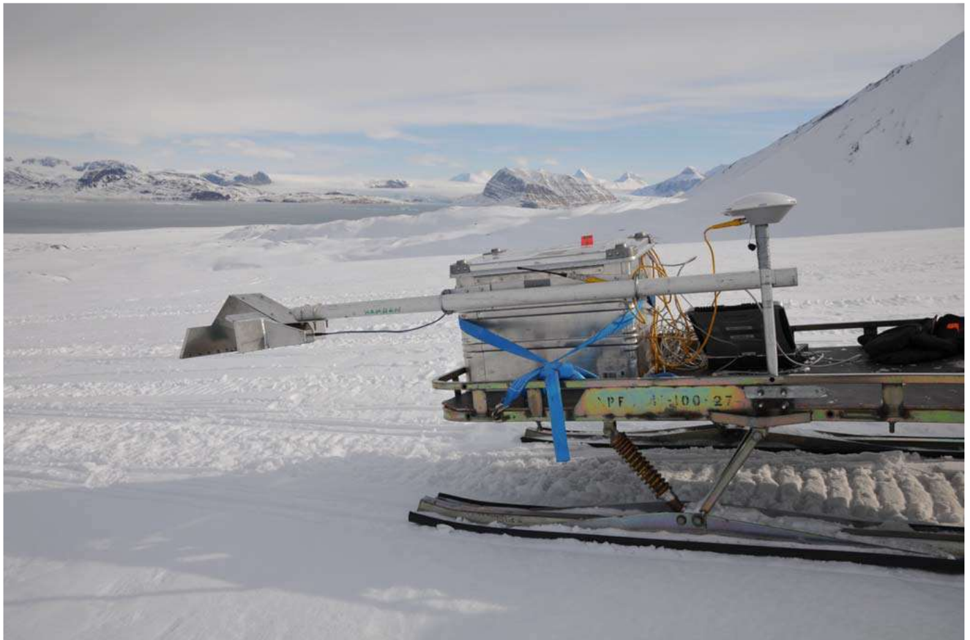
Fig. 4 The photo shows the antenna mounted on a sled at approximately 60 cm above the snow surface.
