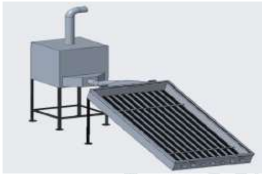
Fig 1 Schematic view of the solar dryer
