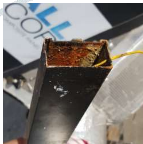
Fig 22 Corrosive effect of FSH material on PCM storage
