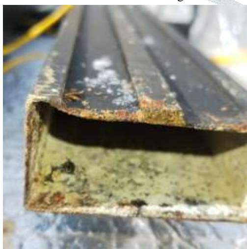
Fig 22 Corrosive effect of FSH material on PCM storage
