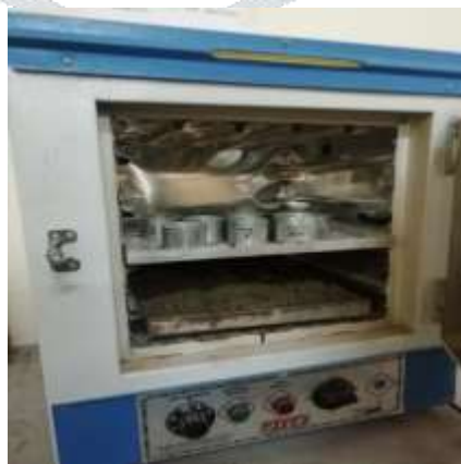
Fig.2. soil sample is dried at a temperature of 105 degree celcius for 24 hrs. in dry oven
