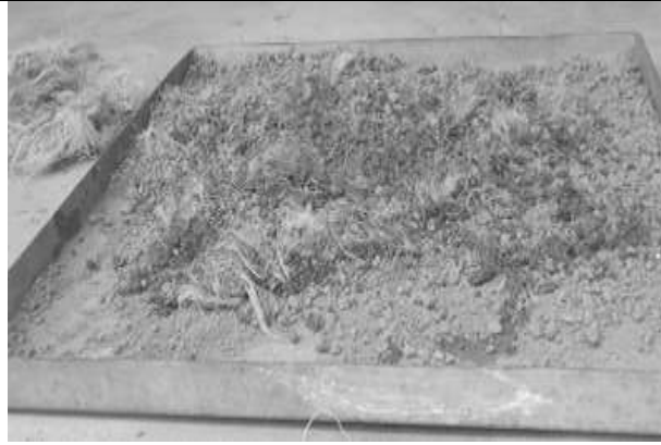
Fig.9 coir Reinforcement with soil.
