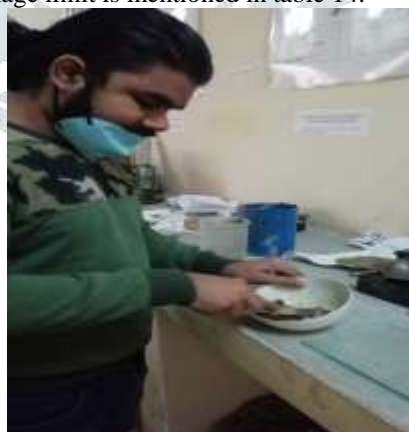
Fig.5. mixing the soil in brass cup during liquid limit test
