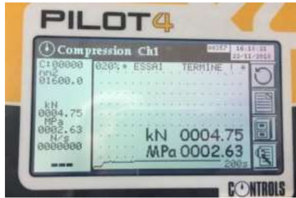
Fig 3 Example of Compressive Strength Testing Result
