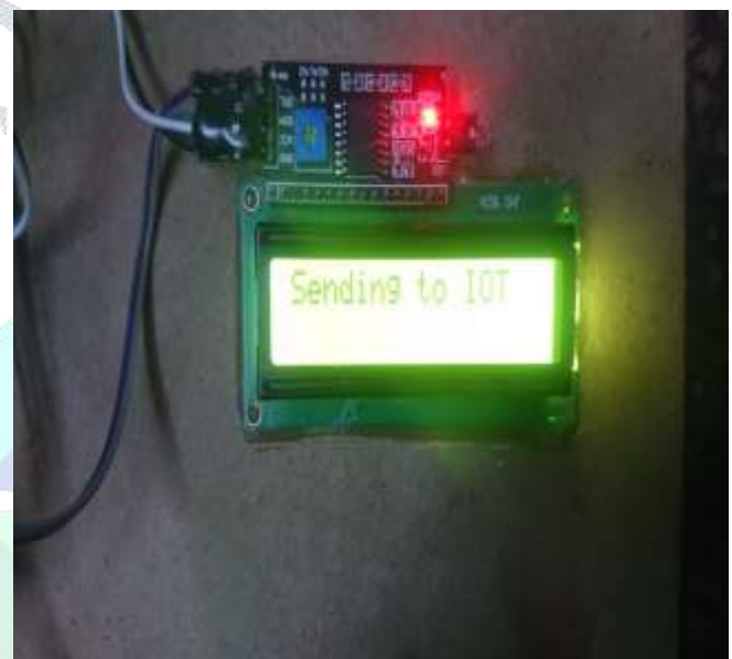
Fig.14 Sensors data sending to Cloud that displayed in LCD
