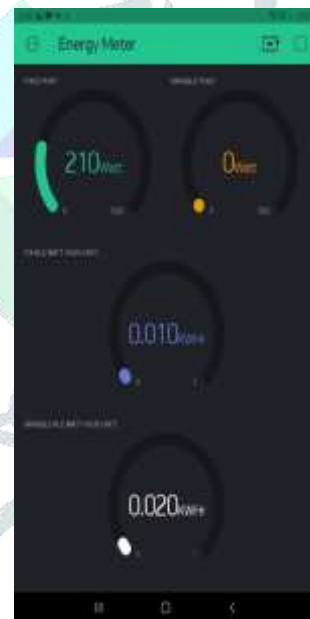
Figure 5: Reading when Load exceeds the power limit
