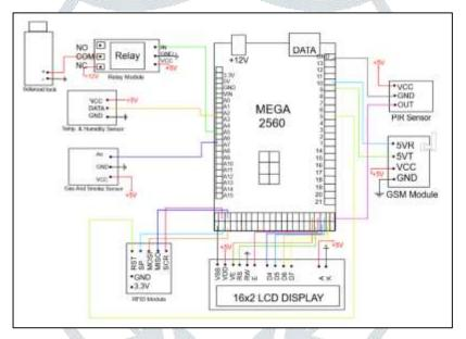
Figure 1: Circuit diagram with all the Connections
