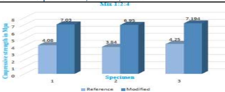
Graph 7: Comparison of compressive strengths of reference mix (1:3:6) with respective modified mix iron ore tailings cured for 7days.
