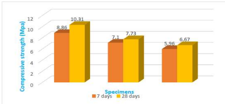
Graph 3: Comparison of compressive strengths of reference mixes cured for 7 and 28 days.
