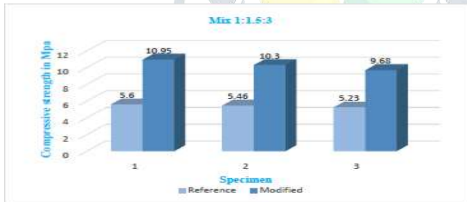
Graph 8: Comparison of compressive strengths of reference mix (1:1.5:3) with respective modified mix iron ore tailings cured for 28 days.
