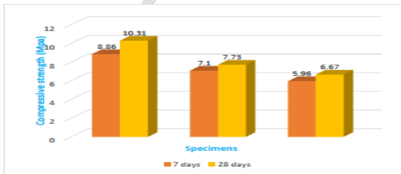
Graph 5: Comparison of compressive strengths of reference mix (1:1.5:3) with respective modified mix iron ore tailings cured for 7 days.
