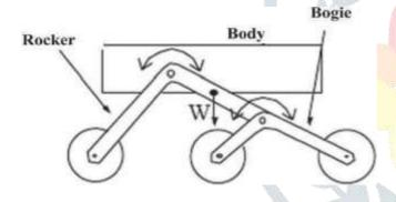
As accordance with the motion to maintain centre of gravity of entire vehicle, when one rocker moves up- ward, the other goes down. The chassis plays vital role to maintain the average pitch angle of both rockers by allowing both rockers to move as per the situation.[4]
