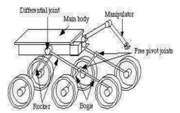
of Rocker Bogie Mechanism
