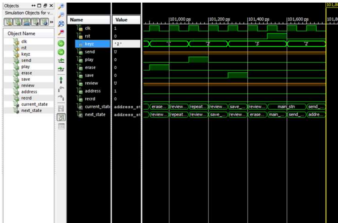
Fig.5. Simulation Result of Voice Message Controller for Secured Communication Figure No.5 demonstrates that the waveform of Voicemail system. It demonstrates how output is change in accordance with the input.
