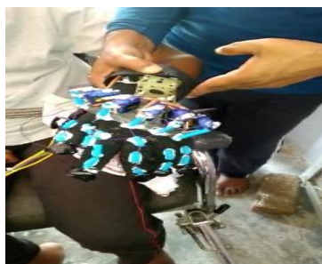
Fig.No.2: Finger Flexion Motion during Rehabilitation through Servo Motor Based Robotic Hand Glove
