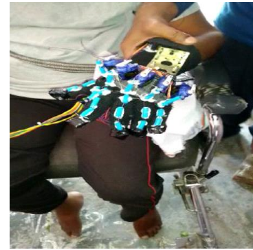
Fig.No.3: Finger Extension Motion during Rehabilitation through Servo Motor Based Robotic Hand Glove
