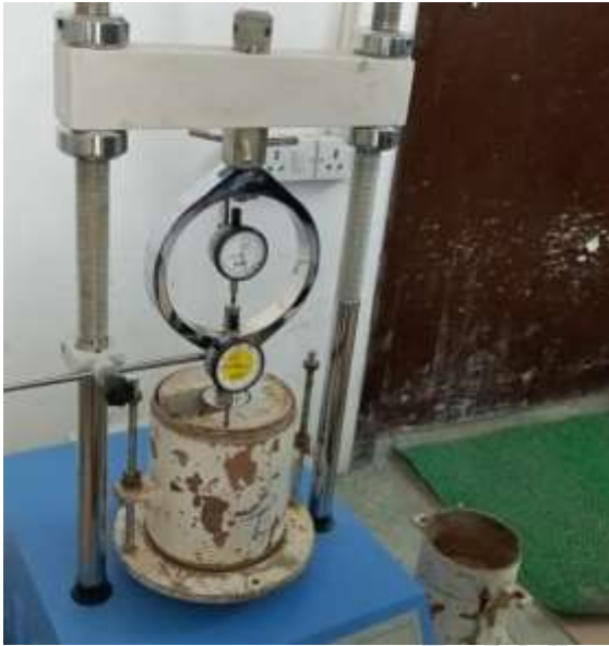
Fig 14. Shows CBR test.
