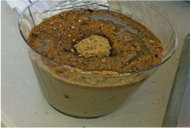
Figure 08:- Exercising the gel strength of a fluid mixture in order to suspend sand for transportation.( Trenchless Technology 2013 )
