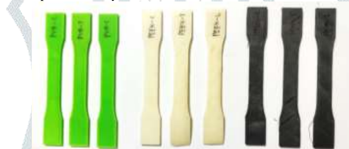
Fig. 8 Shows the line, triangular and concentric set of samples for tensile testing
