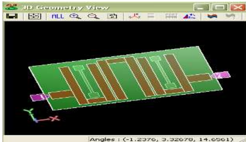
Figure 12. 3-D View of the proposed filter structure
