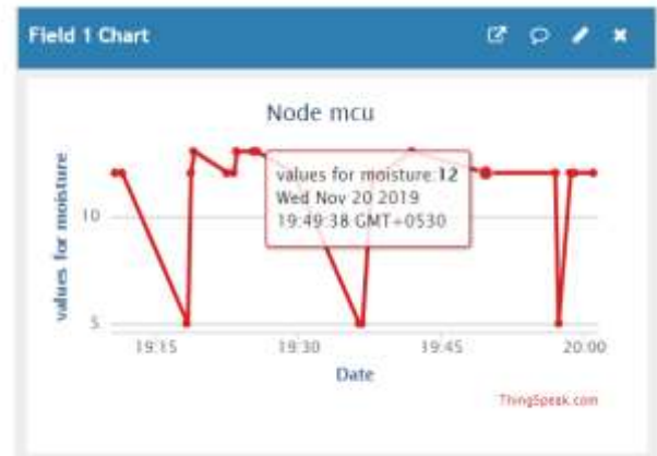
Figure 10: Result of the sensed moisture by sensor
