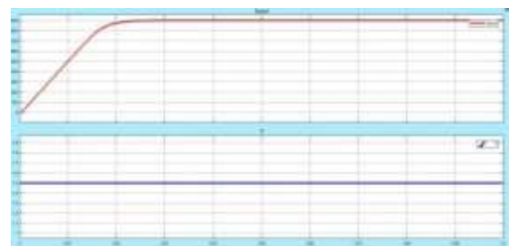
Fig.8. Speed responses of PI Controller reference speed 900rpm at Half load condition
