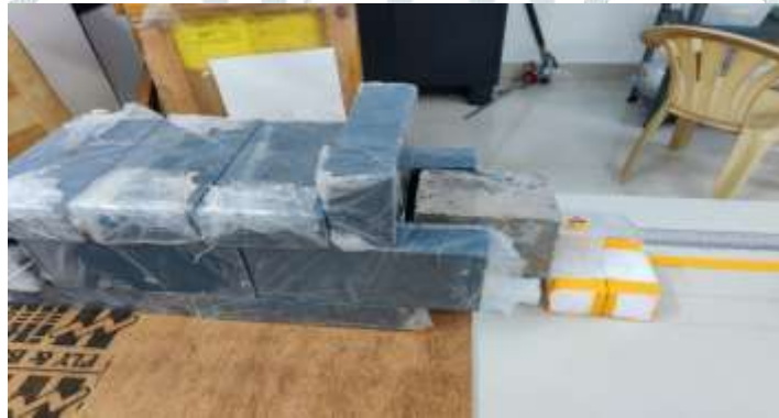
Fig. 2. Gamma Radiation Shielding setup
