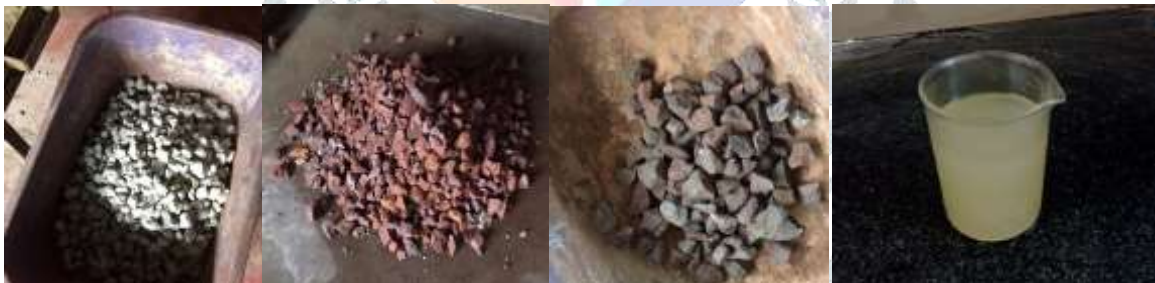
Fig. 1. Coarse aggregate, Hematite, Magnetite aggregates and sodium silicate
