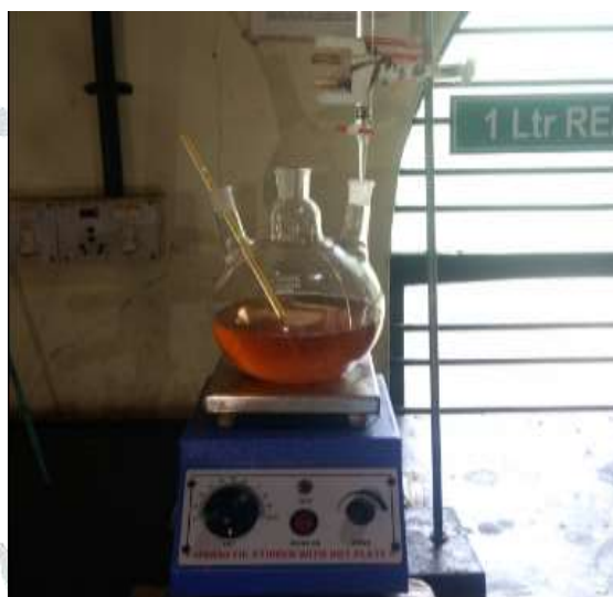
Fig. 1: Apparatus for epoxidation and oxirane ring opening processes.
